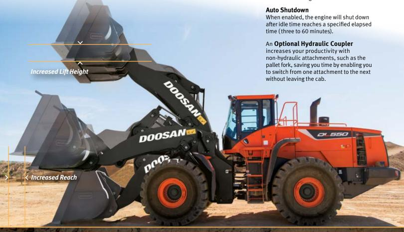
**Z-Bar Lift Arm Linkage** is designed for heavy lifting in loading applications, with geometry that enables rapid bucket movement and proper angle positioning in every situation.
